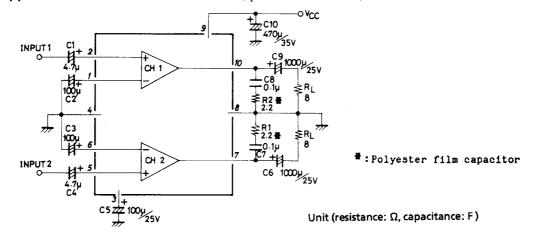
Sample Application Circuit 1 : Dual-channel use (specified Test Circuit)
