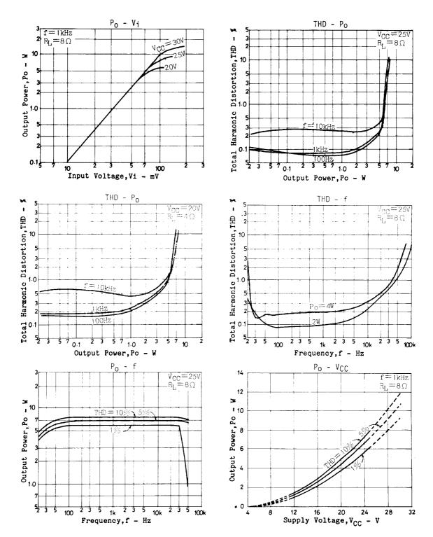
In this application, output capacitors must be used. Since the IC handles an apparent load of  $4\Omega$ , more distortion results, making it impossible for the IC to deliver power at THD=1% as in 2-channel use. It is possible for the IC to deliver power at THD=5% or 10%
